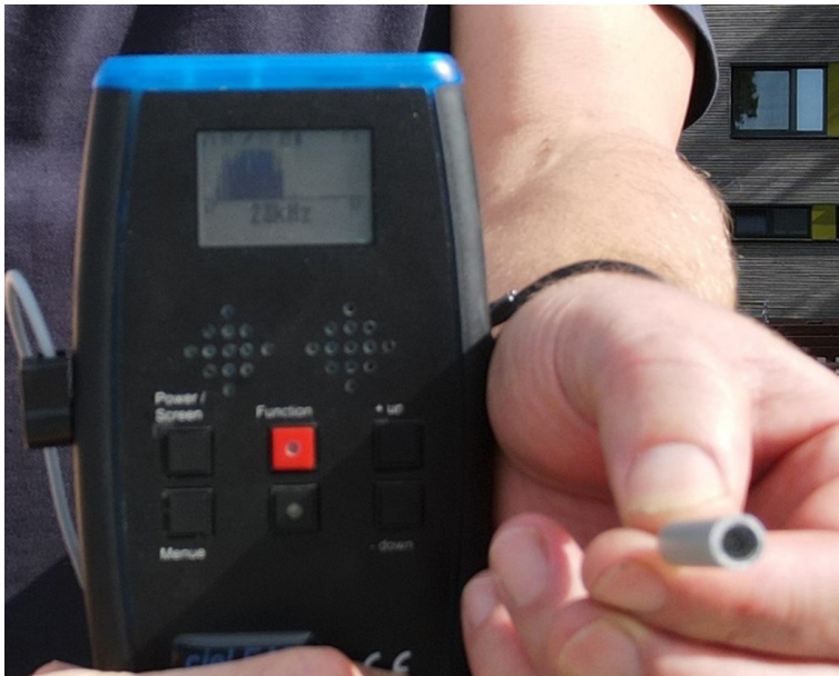
Fig. 12: Reprogrammed bat detector. Displays noises in the frequency range that is above that which is audible to humans and is well perceived by cows (Photo: LBZ Echem)
