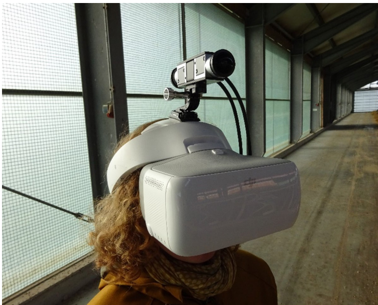
Fig. 11: With the „Echemer cow glasses“ stables can be viewed from the cow’s perspective. In particular, the all-round view, the low visual acuity and the heavily delayed light and dark adaptation provide information about an adapted handling of the animals (Photo: LBZ Echem)
